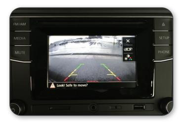
NOTICE: The rear camera visualization will not happen if the trunk is open. Make sure that the trunk is closed through the functioning tests.
